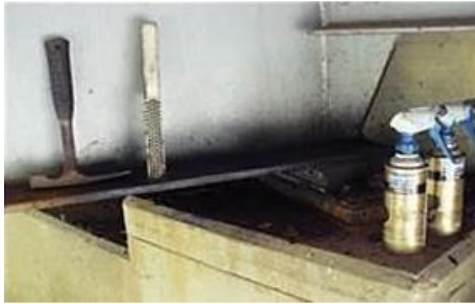
Figure A.5 Penetrating Spray Grease Used on Bearings (Courtesy of PennDOT)
