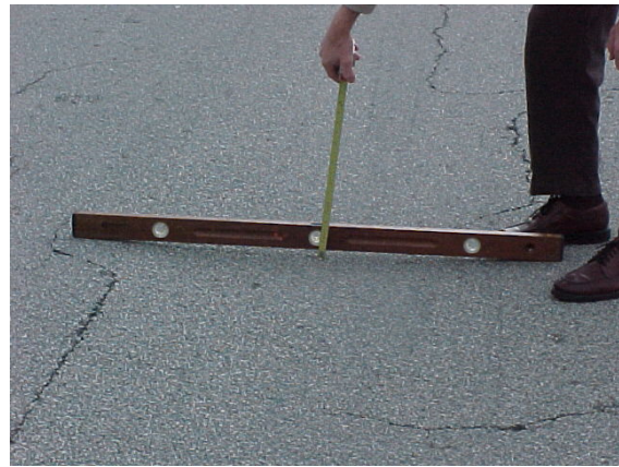
Measuring the depth of a depression.
