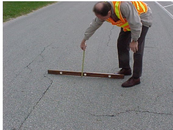
Measuring the depth of a depression.
