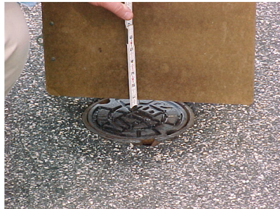
Depression at a water valve in pavement.
