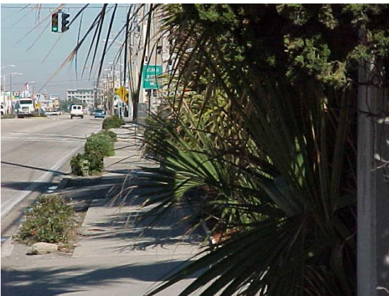
These pictures are examples of vegetation growing over the sidewalk. This obstructs the use of the sidewalk by pedestrians. If there is encroachment of vegetation onto the sidewalk more than 6 inch it does not meet MRP standards.
