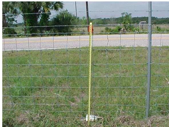
Measure the height of the fence from natural ground to the top of the fence fabric.
