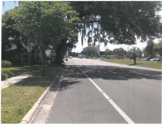
Examples of trees over roadway if measured lower than 14½ feet it would not meet MRP standards.
