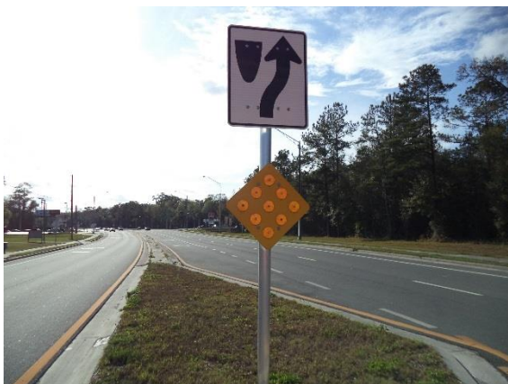
Type 1 (9 button) object marker
