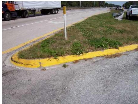
Painted curb markings are rated as symbols. Do not rate curb markings for nighttime reflectivity.
