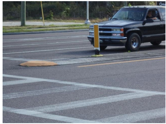
Paddle type, high visibility flexible delineators
