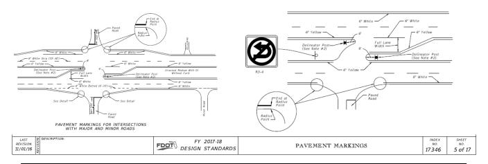
Standard Plans shows the proper placement of delineator posts for median cross-overs and intersections. The horizontal placement of post-mounted delineators at crossovers shall be installed within plus or minus <u>1 foot 6 inches</u> in accordance with the Standard Plans. The index shows the edge of pavement as the standard reference point.
