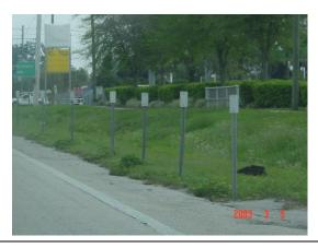
Do not rate post-mounted markers installed to prohibit unauthorized traffic movements (off- tracking, median crossing, shoulder parking, etc.)
