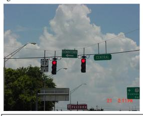
Do not rate county/city signs on signal cables. The US 17 route marker would be rated as a sign >30 sq.ft. because it is an over-lane sign.
