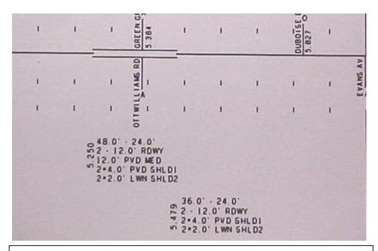
This is an example of a straight line diagram (SLD) that shows 2-4.0' paved shoulders and 2-2.0' lawn shoulders. In this case FLEXIBLE PAVED SHOULDER/TURNOUT and UNPAVED SHOULDER characteristic should be rated.
