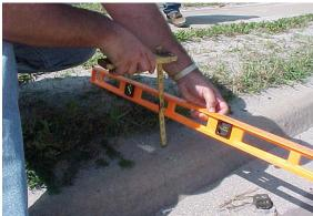
This is a soil buildup greater than 4 inches in the utility strip. It is built up more than 10 continuous feet and, therefore, does not meet MRP standards.
