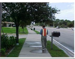
This tree limb appears lower than 8-1/2 feet over the sidewalk. This does not meet MRP standards.
