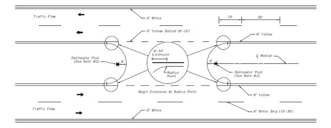
PAVEMENT MARKINGS AND DELINEATORS FOR MEDIAN CROSS-OVER
