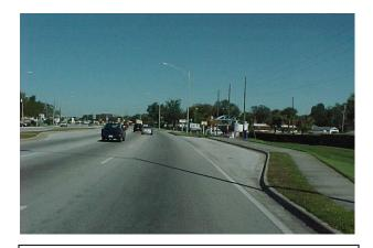
The paved area to the right in this photo is a bus turnout. The pavement in a bus turnout should be evaluated as roadway pavement.
