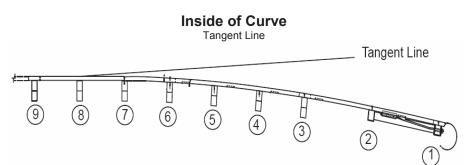
The SRT-350 8 POST<sup>™</sup> system offsets are measured at a tangent line from the start of the SRT-350 8 POST<sup>™</sup> system. If an offset places a post on the shoulder, then the face of the rail must be on the edge of the shoulder for that offset.
