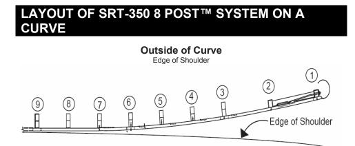
The SRT-350 8 POST™ system offsets are measured at the edge of shoulder from the start of the SRT-350 8 POST™ system.
