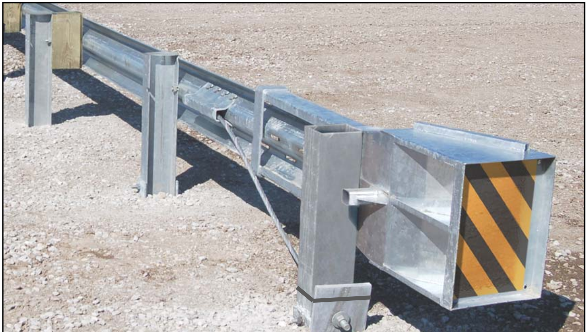
Figure 5. View of FLEAT-SP-MGS Steel End Post #1
