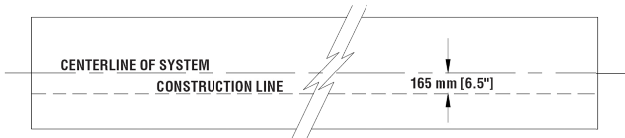
Figure 14 (Top view of concrete foundation)
