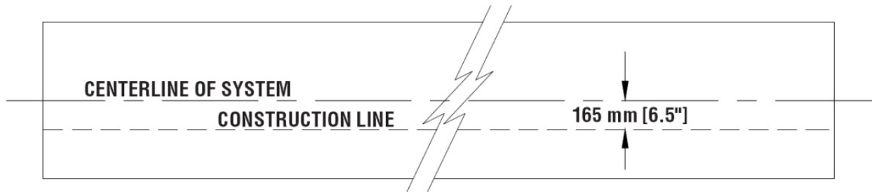
Figure 15 (Top view of concrete foundation)
