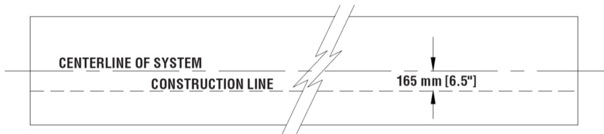
Figure 46 (Top view of concrete foundation)
