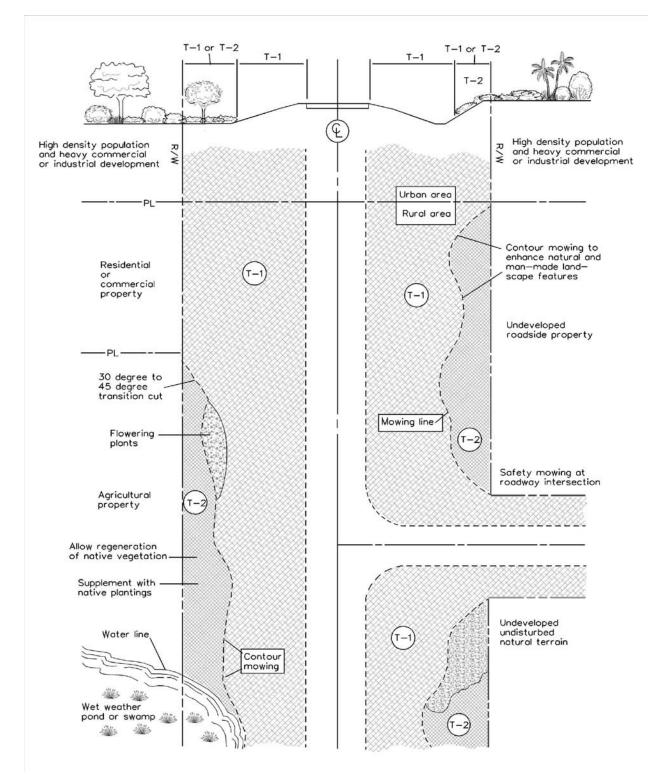
Figure 18. Mowing Plan (Arterial Roads Only)
