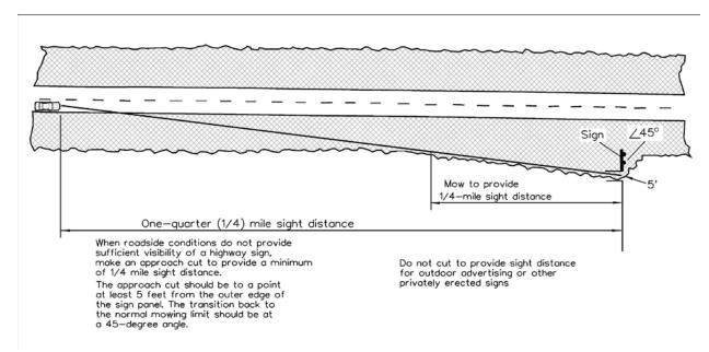
Figure 23. Highway sign mowing limits.
