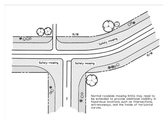
Figure 24. Safety mowing limits.
