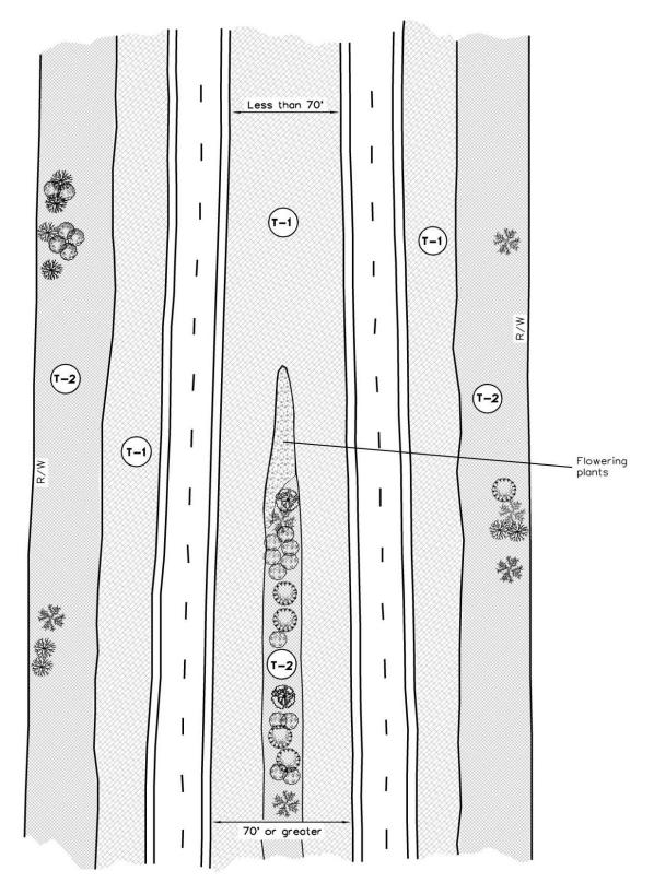
Figure 20. Median mowing limits: Rural arterial and all limited access (overhead view).
