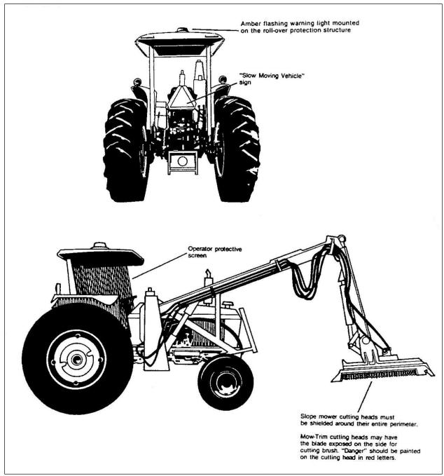
Figure 33. Slope mower safety devices.
