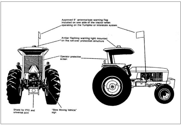
Figure 30. Tractor safety devices.
