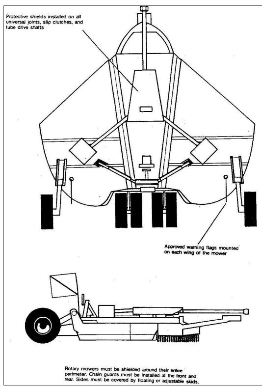
Figure 31. Rotary mower safety devices.
