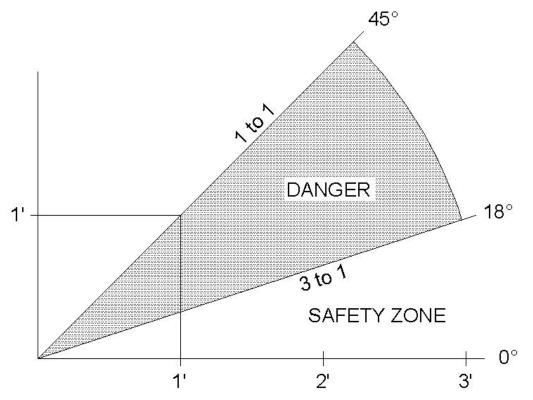
Figure 29. Slope hazards.
