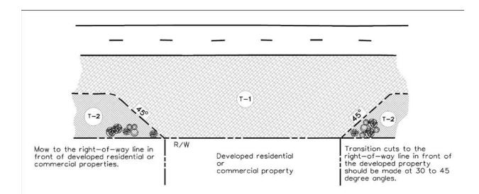
Figure 25. Developed property mowing limits: Rural (arterial roads only).
