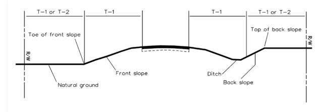
Figure 17. Roadside mowing: Typical section.
