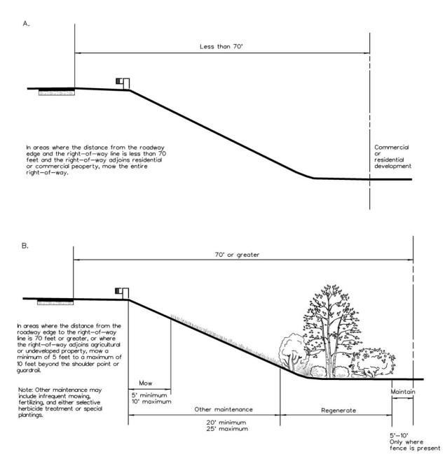
Figure 21. Slope mowing limits: Rural arterial and all limited access.
