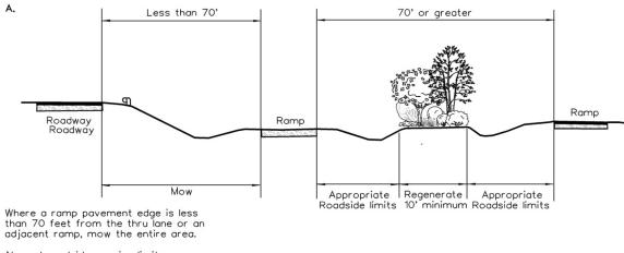
Normal roadside mowing limits should be maintained between ramps of equal elevation.
