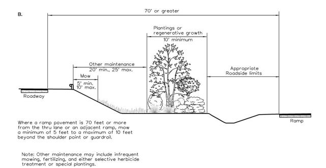
Figure 26. Grade separations and interchange infields: Rural (cross-sectional views).
