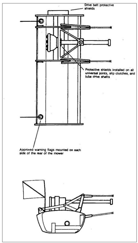
Figure 32. Flail mower safety devices.
