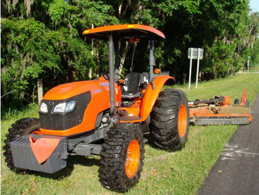
Figure 14. Rotary mower used for mowing along rights-of-way.
