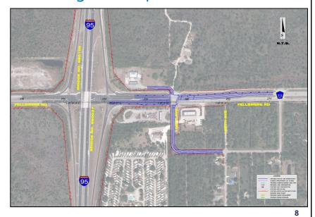
The interchange at Fellsmere Road is expected to operate acceptably through 2045. No interchange or ramp improvements are needed. However, additional turn lanes have been identified at 108 Avenue as an improvement in 2045 to address future intersection capacity deficiencies.
