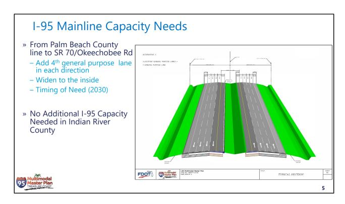
The analysis of the I-95 mainline revealed future volumes will exceed the capacity of the current six-lane freeway by the 2030s. Therefore, a fourth general purpose lane is needed on I-95 from the Palm Beach/Martin county line to SR 70 in St. Lucie County.
