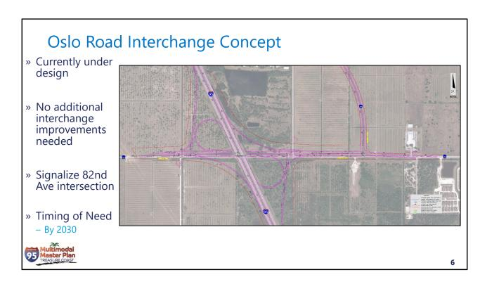
The Oslo Road interchange is currently under design and is expected to be constructed in the mid-2020s. Analysis confirmed that the interchange configuration will operate well as designed through 2045 with no modifications.
