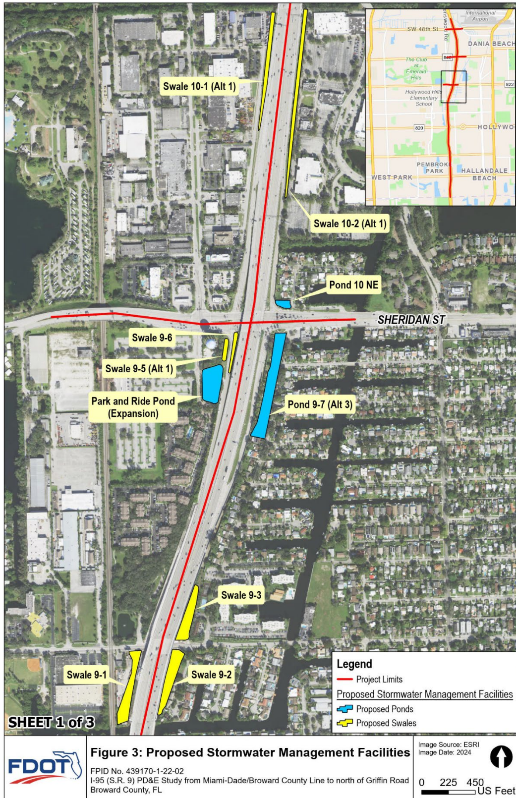
FIGURE 3: PROPOSED STORMWATER MANAGEMENT FACILITIES
