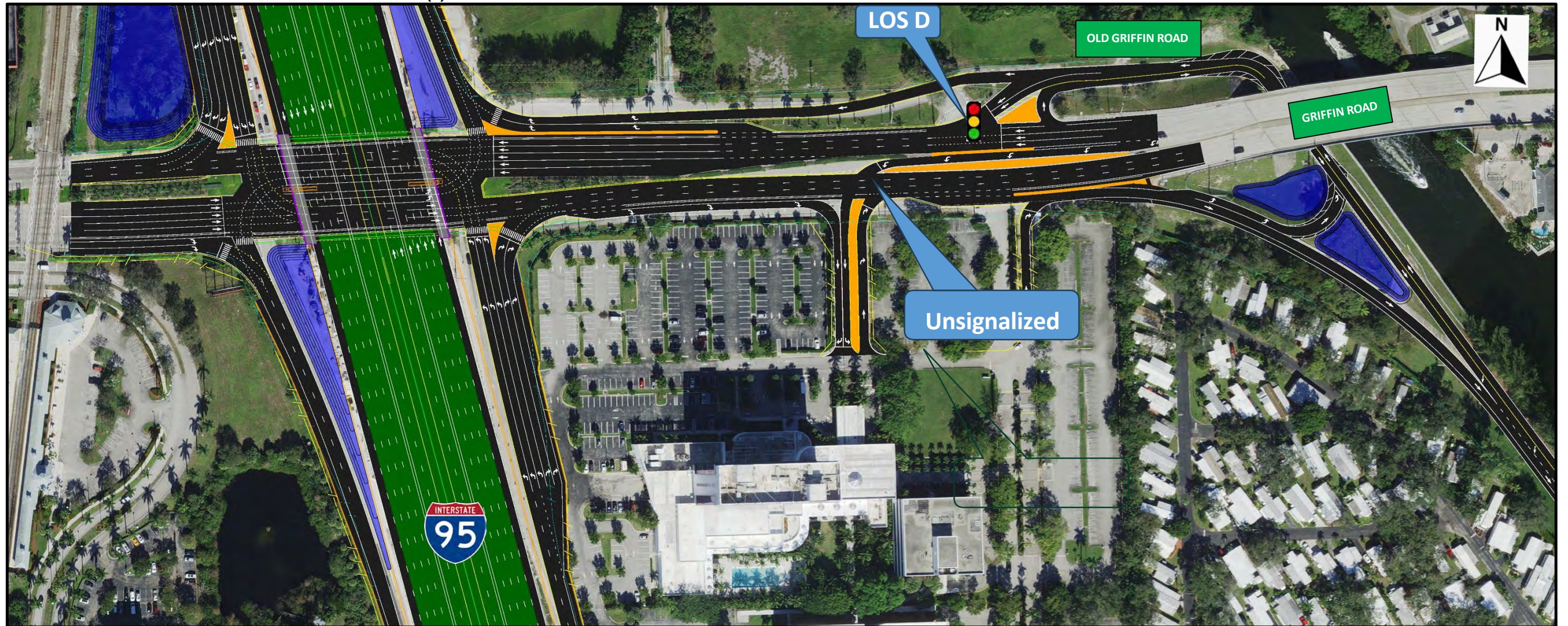
FIGURE 5-6(a): GRIFFIN ROAD AT OLD GRIFFIN ROAD INTERSECTION – ALTERNATIVE A: FREE FLOW EASTBOUND
