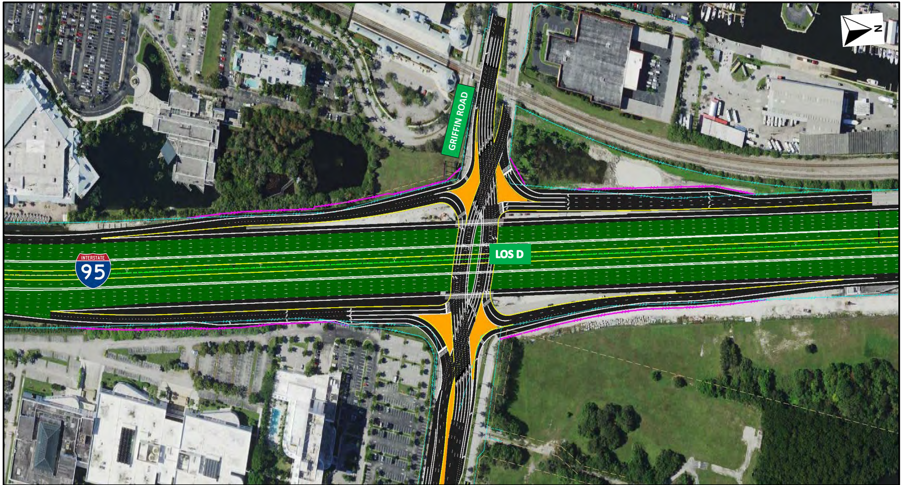
FIGURE 5-5(b): I-95 AT GRIFFIN ROAD INTERCHANGE – ALTERNATIVE B: DIVERGING DIAMOND INTERCHANGE (DDI)
