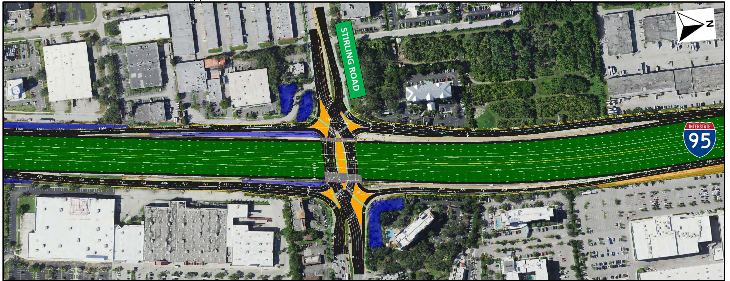
FIGURE 5-4(b): I-95 AT STIRLING ROAD INTERCHANGE – ALTERNATIVE A: DIVERGING DIAMOND INTERCHANGE (DDI)
