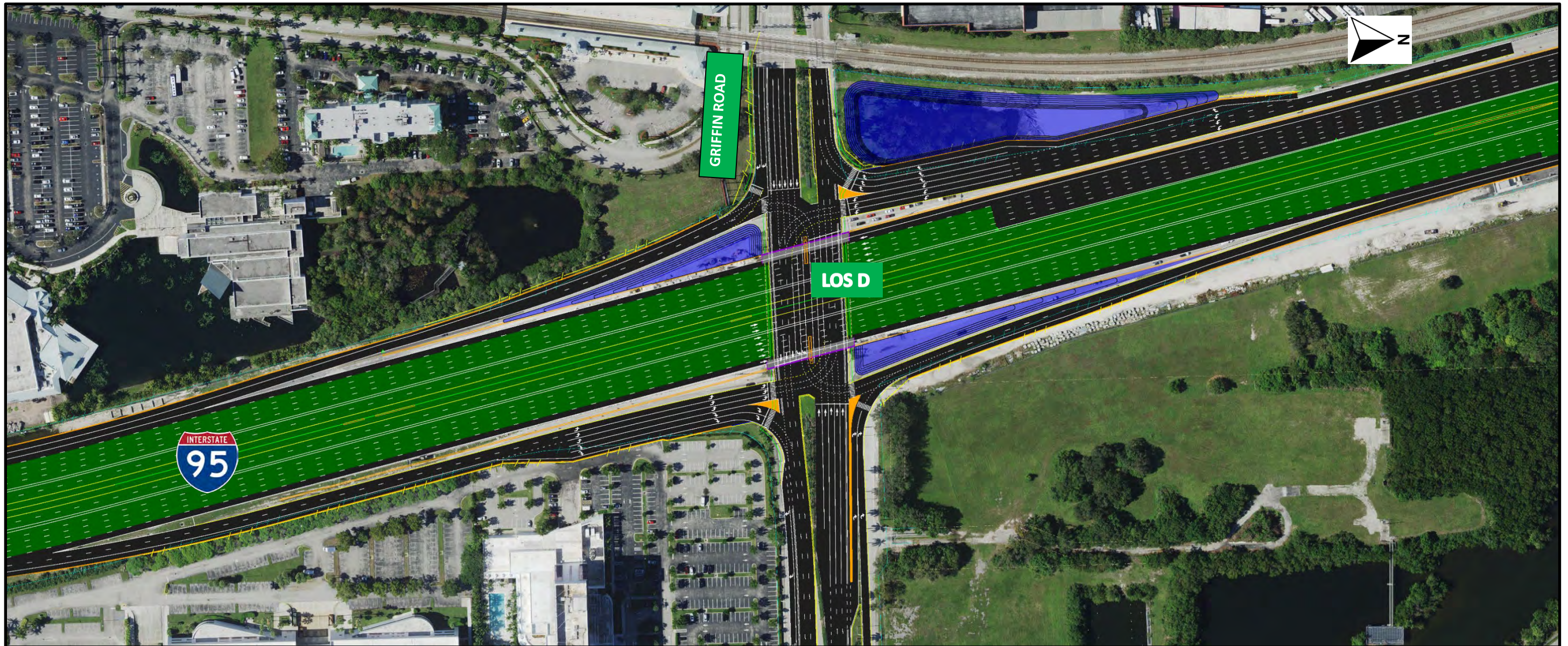
FIGURE 5-5(a): I-95 AT GRIFFIN ROAD INTERCHANGE – ALTERNATIVE A: DIAMOND INTERCHANGE (MODIFY EXISTING)
