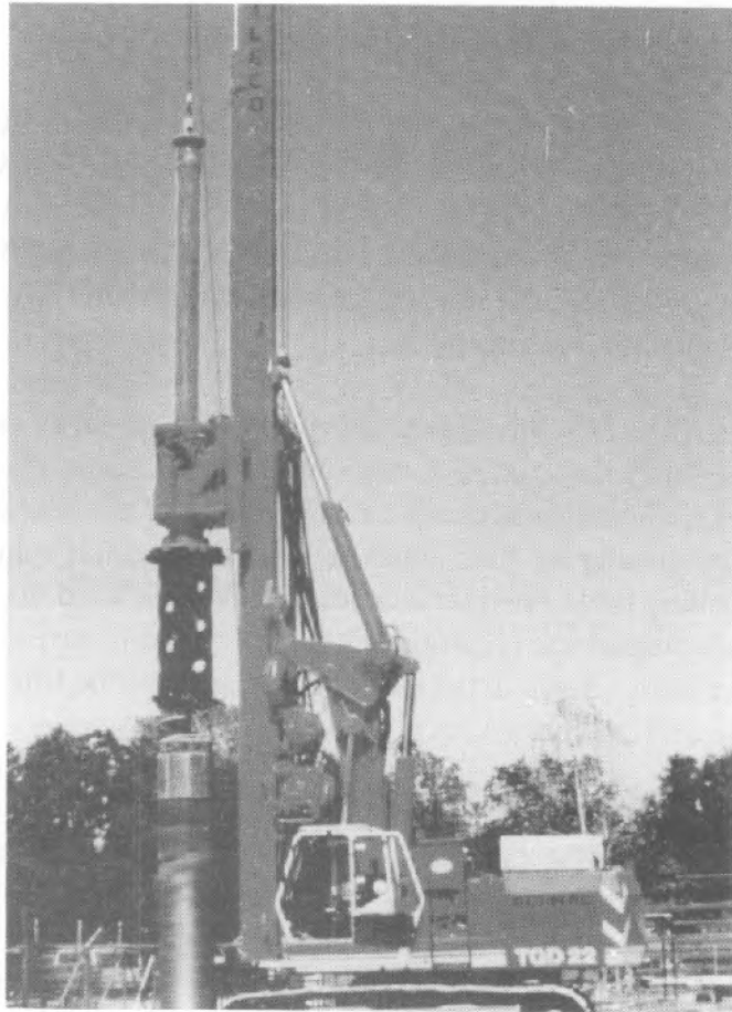
Figure 3.5. Case-and-drill (full-depth-casing) rigs: (a) track-mounted rig with auger
