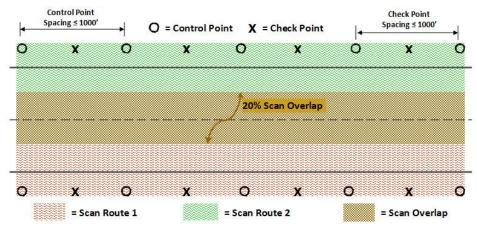
Note: Since all projects are different, these are only recommendations. The Surveyor & Mapper in responsible charge of the TML must choose the appropriate accuracy and geometry of the project control points and checkpoints to ensure the TML survey data and products meet or surpass accuracy requirements of the project.
