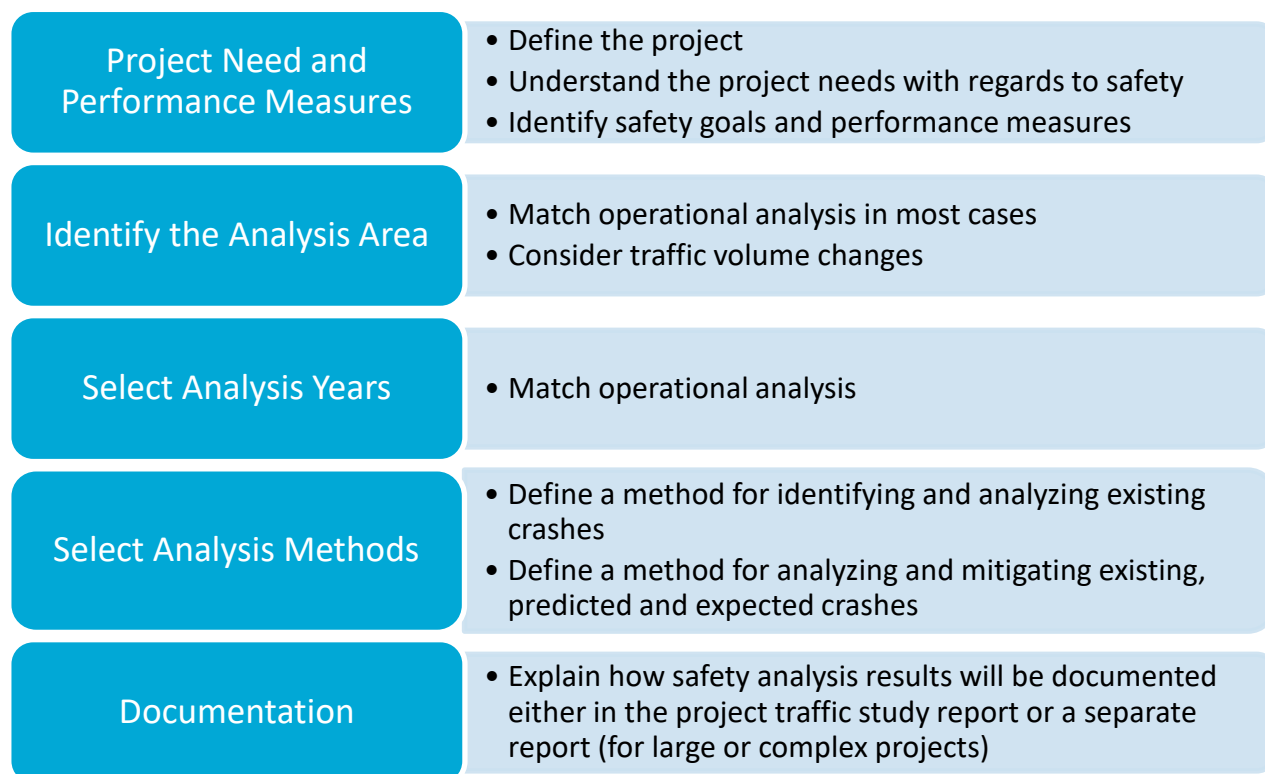
Figure 1 Safety Analysis Scoping Process
