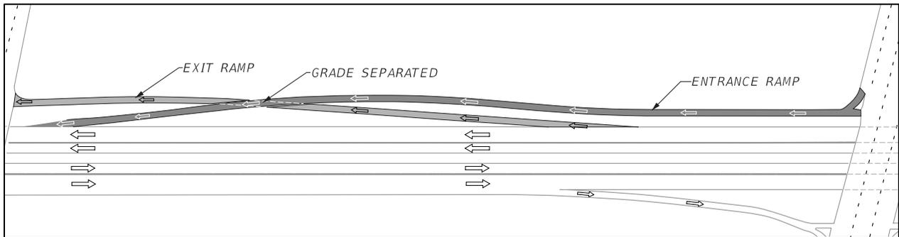
When combining general use lane or general toll lane exits and managed lane exits in a braided ramp configuration, the managed lane exit merges on the right side of the general use lanes or general toll lanes as illustrated in **Figure 211.12.3**. Operational analysis determines the actual lane configuration. Refer to **Traffic Analysis Handbook** and **Interchange Access Request User's Guide** for guidance on analysis requirements.
