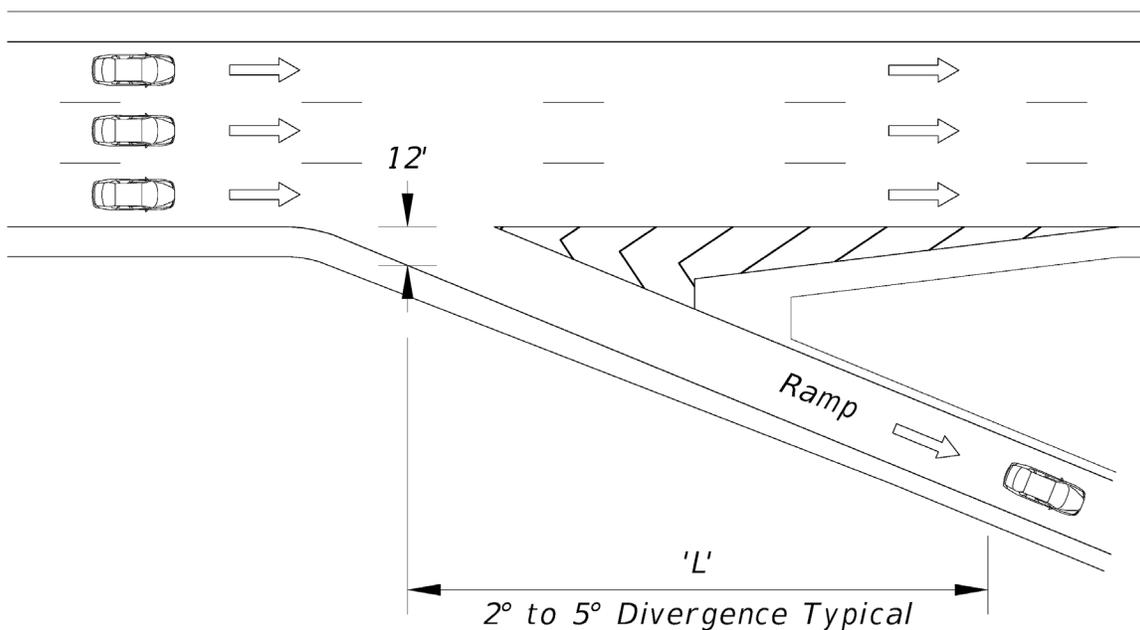
For two lane exit type ramp terminals, it is usually appropriate to develop an auxiliary lane upstream from the exit. A length of 1,500 ft is recommended to develop the full capacity of a two-lane exit. As with single lane exits, attention should be given to obtaining the appropriate deceleration distance between the exit and first horizontal curve on the ramp. See **Figure 211.13.1**. Typical design for two-lane taper type exit terminals is shown in **Figure 211.13.3** below.
