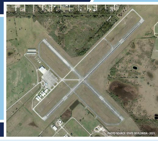
Okeechobee County Airport (OBE) is a general aviation (GA) airport located directly northwest of the City of Okeechobee. The airport provides two intersecting paved runways, the longest of which (Runway 5-23) is 5,000 feet long by 100 feet wide.
