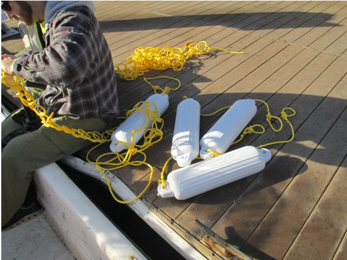
Figure A-16. Small plastic buoys and student coiling anchor lines using daisy chains
