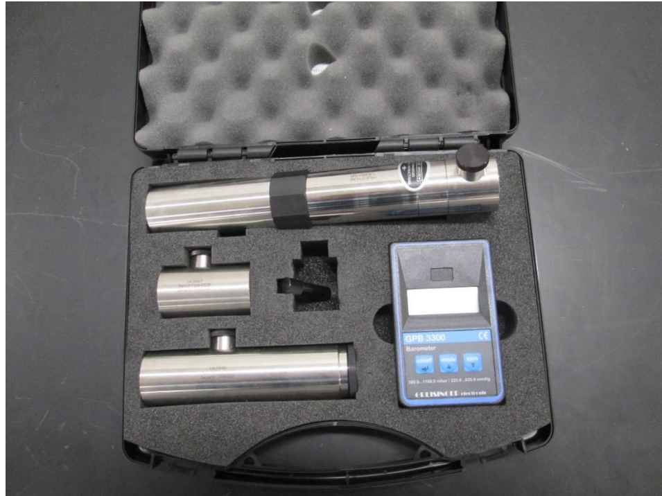
Figure A-4. Calibrator with hydrophone receiver attachment
