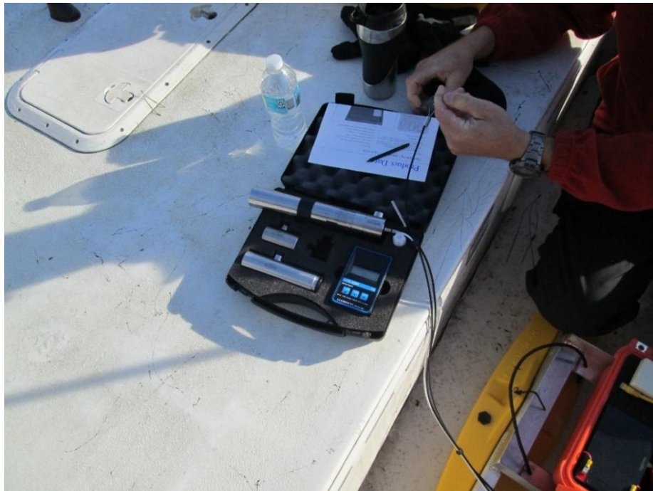
Figure A-6. Hydrophone inserted into calibrator
