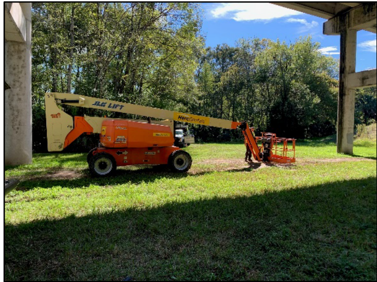
PHOTO 19 - Specialized Equipment, Boom Lift (Ocklawaha River Bridge).
