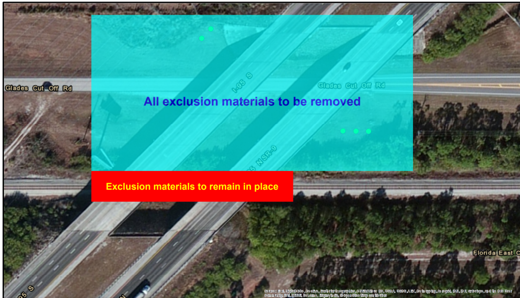
FIGURE 16 - Area over railroad tracks permanently excluded to avoid future safety concerns and ROW conflicts. Citation - Fly-By-Night , I-95 and Glades Cut Off Rd., District Four.
