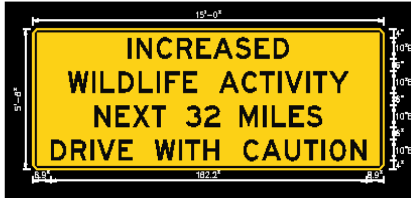
Figure 48 Example of a static sign used in combination with dynamic message signs (DMS) triggered by signals from a wildlife collision-avoidance system (WCAS).
