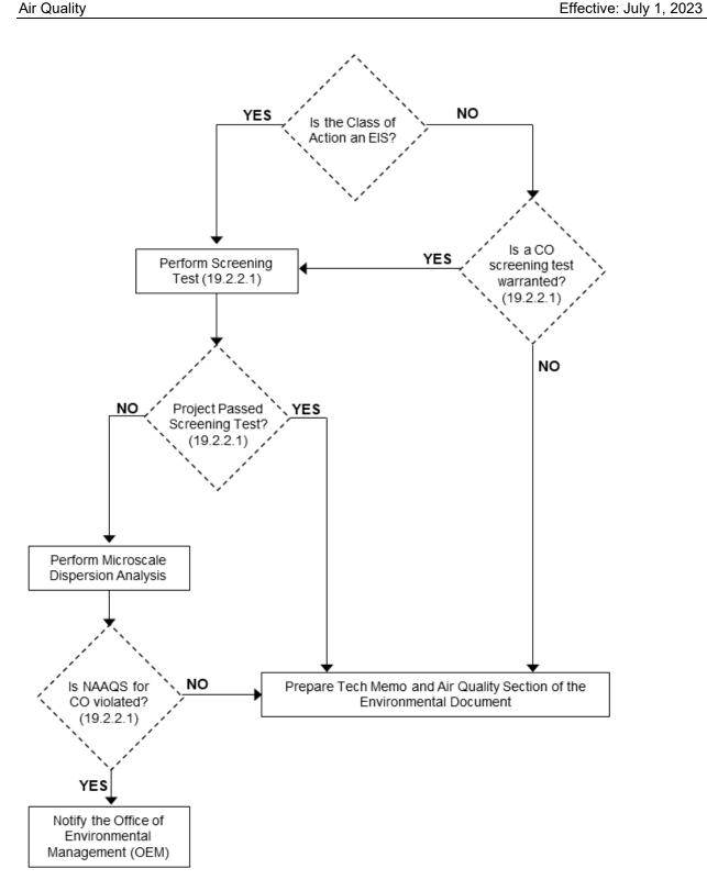
Figure 19-6 Air Quality Analysis Process for Carbon Monoxide
