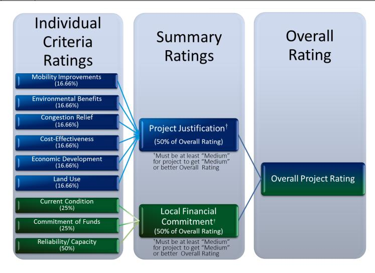
Figure 14-5 New Starts, Core Capacity, and Small Starts Project Evaluation and Rating
