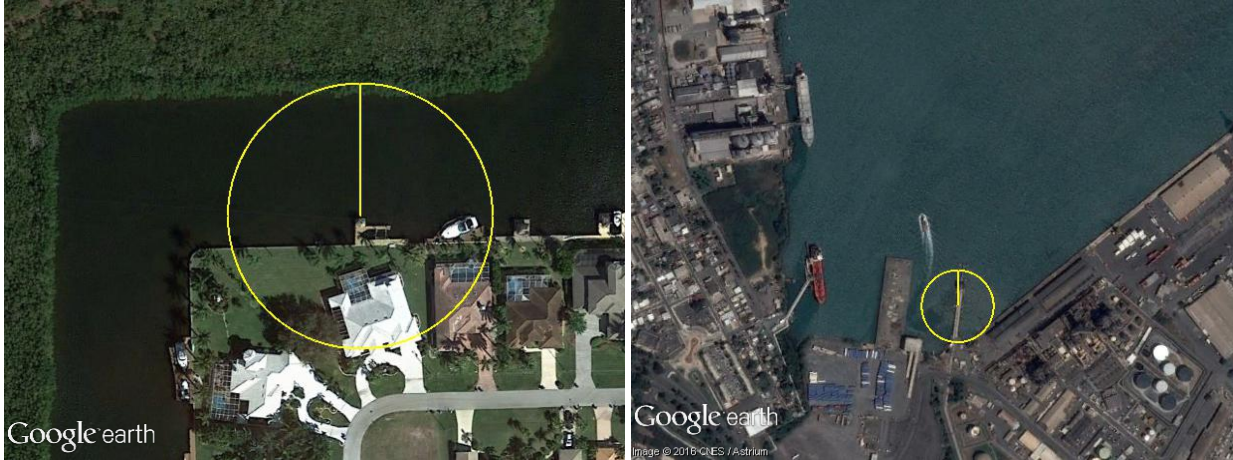
Figure 8. Example of a confined space (left) and an open-water environment (right) for a noise analysis. The left image shows a man-made residential canal and a 150 ft sound radius that would block movement of species if piles were installed at this location because the canal is not wide enough to ensure more than half the escape route is free from cumulative injurious noise levels. The right image shows a portion of San Juan Harbor and a 260 ft sound radius that would not block movement of species if piles were installed at this location because species would be able to move freely away without passing through the area with cumulative injurious noise levels.
