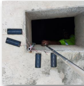
Panels mounted on the underside of bridge
