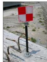
Optical targets with theodolite (Cook-2005)
