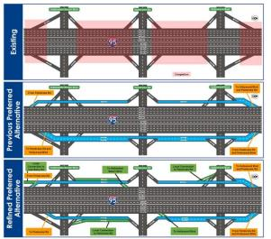
Various design configurations are placed into the model network to test the effectiveness of each design schematic.
