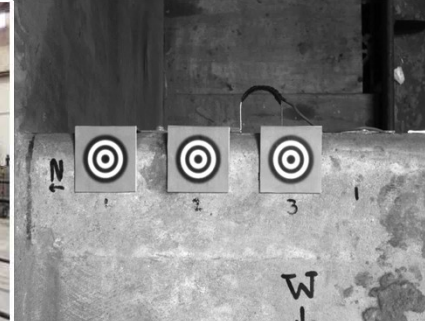
CRACK OPENING TRACKING BY IMETRUM CAMERA
