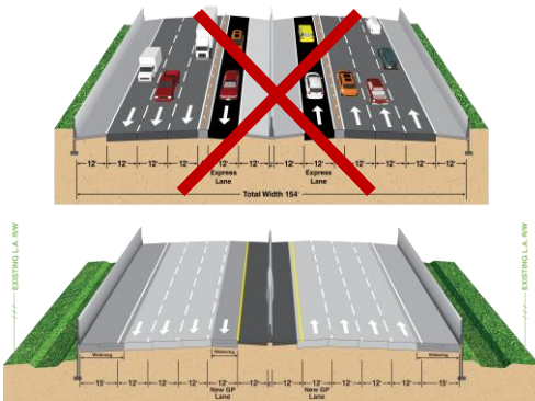
Constructed additional GP lane and accommodated transit – within existing ROW
