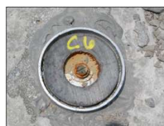
Optical targets with theodolite
