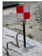
Optical targets with theodolite
