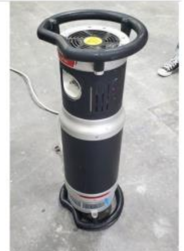
Portable YXLON X-Ray machine
