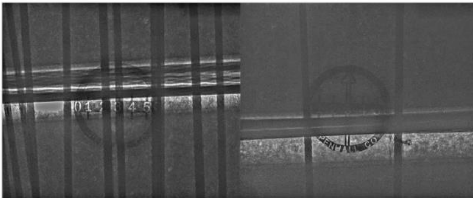
Internal Duct Specimen: duct with strands
