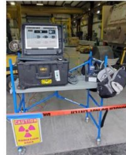
Portable YXLON X-Ray machine
