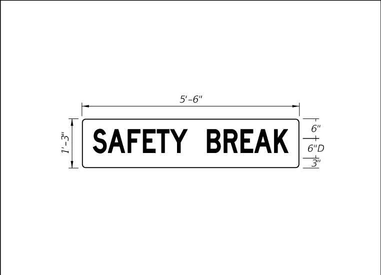
FTP-411-25 5'-6" X 1'-3" 3" Radii ¾" Border 6" Series D Legend Blue Background White Legend and Border
