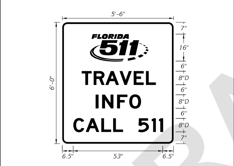
FTP-414A-25 5'-6" X 6'-0" 3" Radii 1" Border 8" Series D Legend Blue Background White Legend and Border
