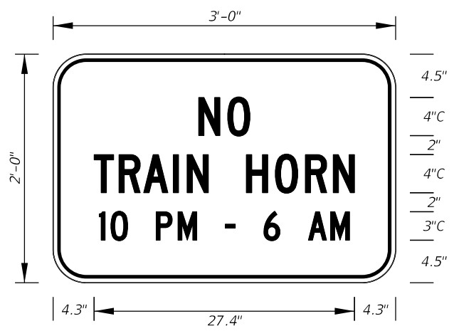
FTP-203-25 3'-0" X 2'-0" 1.5" Radii 3/4" Border 4" and 3" Series C Legend Yellow Background Black Legend and Border
