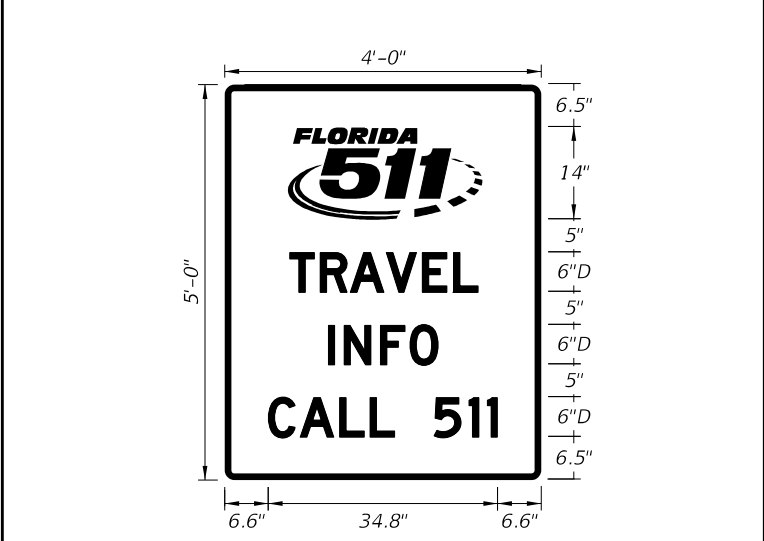
FTP-414-25 4'-0" X 5'-0" 3" Radii 1" Border 6" Series D Legend Blue Background White Legend and Border
