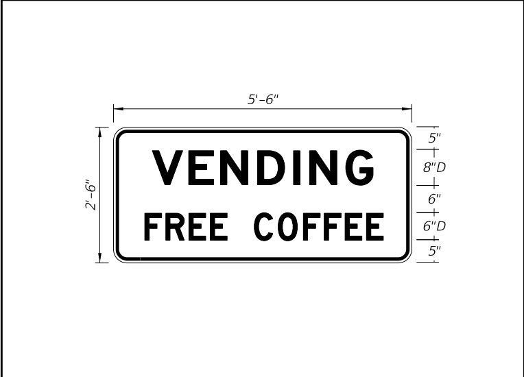
FTP-410-25 5'-6" X 2'-6" 3" Radii ¾" Border 8" and 6" Series D Legend Blue Background White Legend and Border
