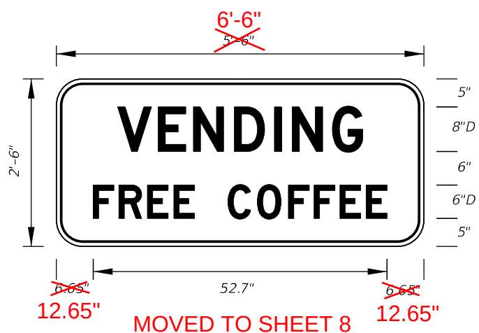
FTP-74-06 5'-6" X 2'-6" 4" Radii \frac{3}{4} " Border 6" Series D Legend Blue Background White Legend and Border
