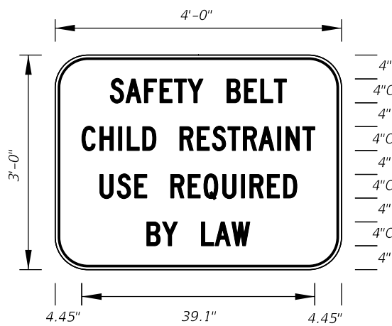
FTP-44A-25 4' X 3' 5" Radii 3/4" Border 4" Series C Legend White Background Black Legend and Border
