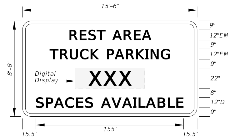
FTP-87-21 15'-6" X 8'-6" 12" Radii 2" Border Series D Legend Series EM Legend Blue Background White Legend and Border
