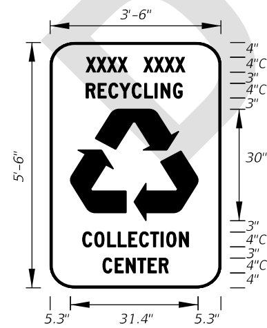
FTP-49-06 3'-6" X 5'-6" 6" Radii 4" Series C Legend Green Background White Legend, Border and Symbol Municipality Name Optional
