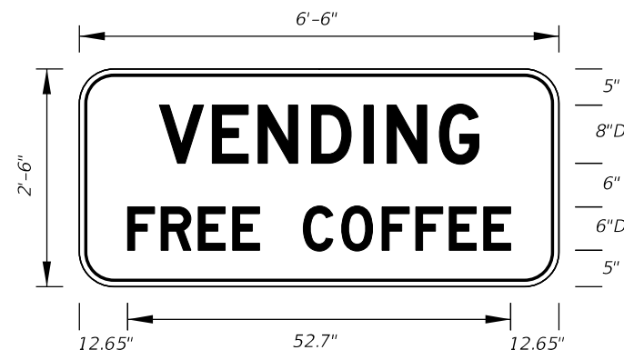
FTP-74-06 6'-6" X 2'-6" 4" Radii 3/4" Border 6" Series D Legend Blue Background White Legend and Border
