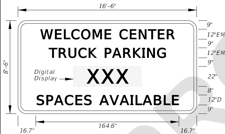
FTP-89-21 16'-6" X 8'-6" 12" Radii 2" Border Series D Legend Series EM Legend Blue Background White Legend and Border
