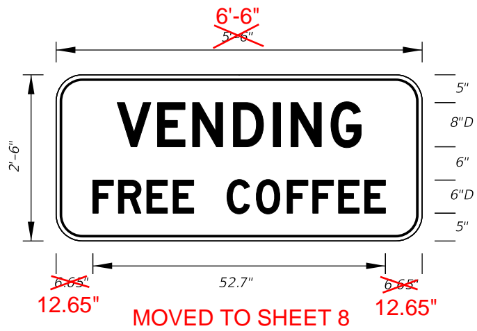
FTP-74-06 5'-6" X 2'-6" 4" Radii 3/4" Border 6" Series D Legend Blue Background White Legend and Border
