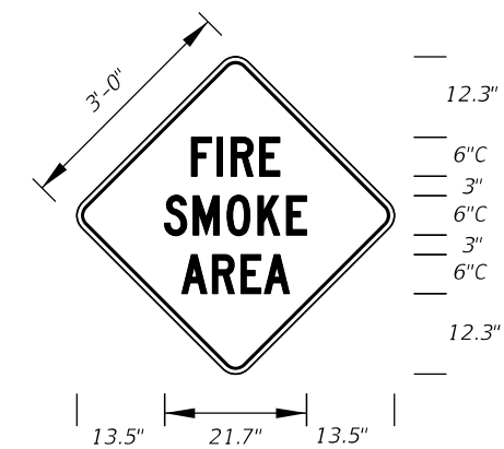
FTP-72-06 3' X 3' 2" Radii 3/4" Border 6" Series C Legend Yellow Background Black Legend and Border
