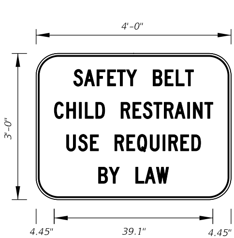
FTP-44A-25 FTP-45-06 4' X 3' 5" Radii 3/4" Border 4" Series C Legend White Background Black Legend and Border
