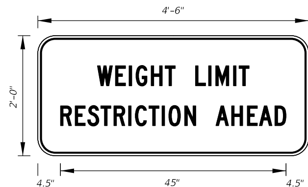
FTP-50-06 4'-6" X 2' 3" Radii 3/4" Border 4" Series C Legend Yellow Background Black Legend and Border
