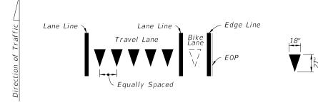
Yield Lines consist of five - 18" X 27" white triangles which face traffic. Equally space triangles within traffic lane. When a bike lane is present, add one additional triangle in the center of the bike lane.
