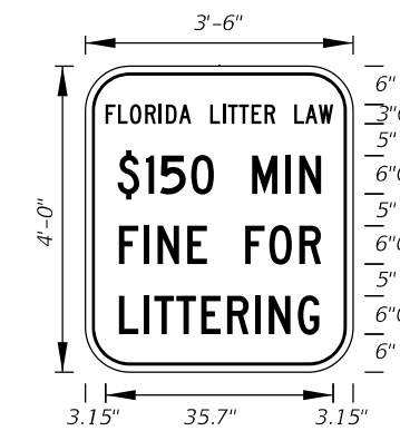
FTP-40-21 3'-6" X 4' 6" Radii 3/4" Border 3" and 6" Series C Legend White Background Black Legend and Border
