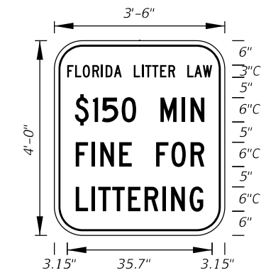
FTP-40-21 3'-6" X 4' 6" Radii 3/4" Border 3" and 6" Series C Legend White Background Black Legend and Border
