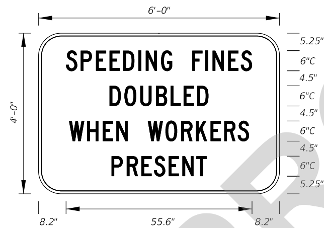
MOT-13-06 Freeway Sign 6' X 4' 6" Radii 3/4" Border 6" Series C Legend White Background Black Legend and Border
