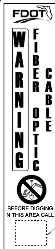
FIBER OPTIC CABLE ROUTE MARKER LABEL DETAIL
