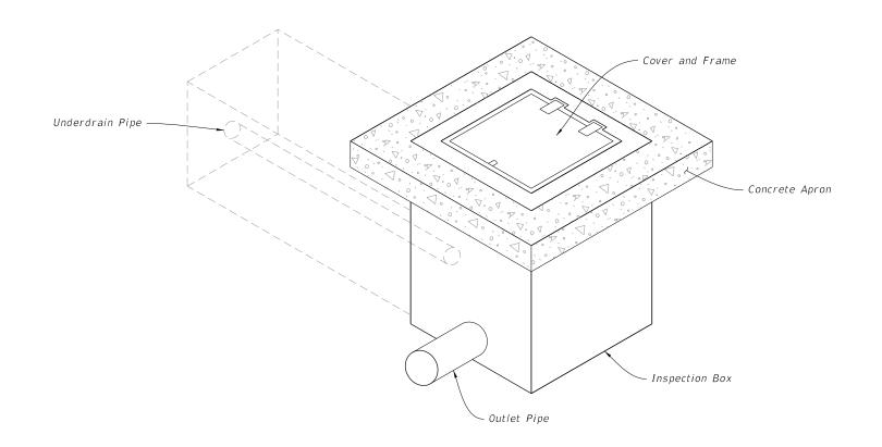
=UNDERDRAIN INSPECTION BOX ASSEMBLY ===
