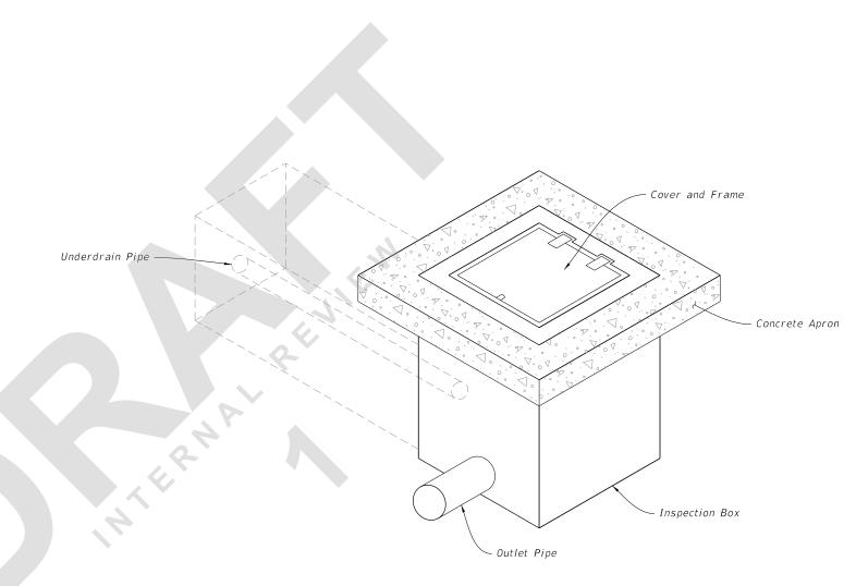
=UNDERDRAIN INSPECTION BOX ASSEMBLY ===
