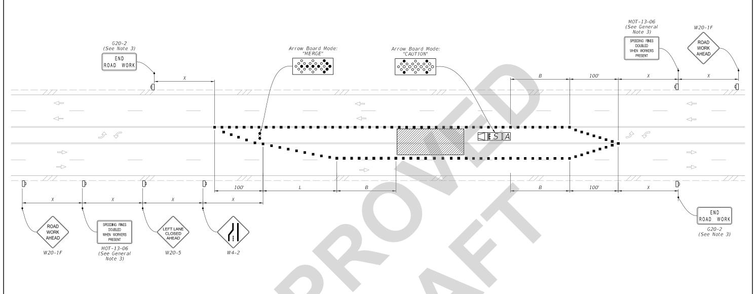
TEMPORARY MULTILANE, TWO-WAY LEFT-TURN LANE, TURN LANE CLOSURE= (Closure of One Inside Lane Shown, Closure of both Similar)
