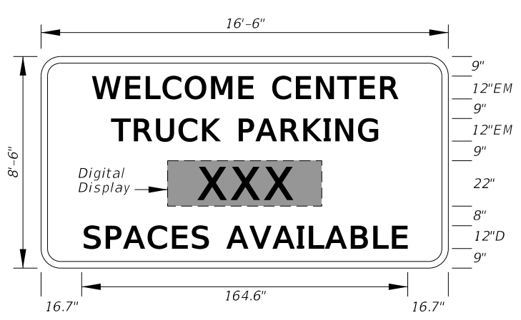
FTP-89-21 15'-6" x 8'-6" 12" Radii 2" Border Series D Legend Series EM Legend Blue Background White Legend and Border
