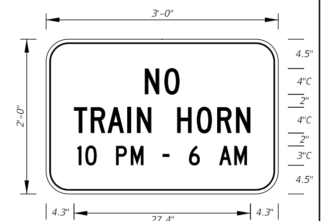
FTP-61-06 3' X 2' 3" Radii 3/4" Border 4" and 3" Series C Legend Yellow Background Black Legend and Border
