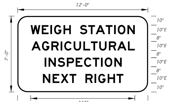
FTP-7A-06 12' X 7' 11" Radii 2" Border 10" Series E Legend Green Background White Legend and Border
