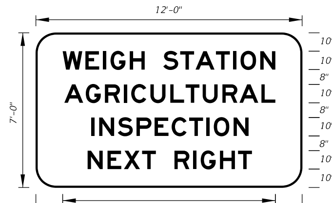
FTP-7A-06 12' X 7' 11" Radii 2" Border 10" Series E Legend Green Background White Legend and Border
