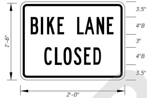
MOT-25-21 2'-0" x 1'-6" 1.5" Radii 1/2" Border 4" Series B Legend White Background Black Legend and Border
