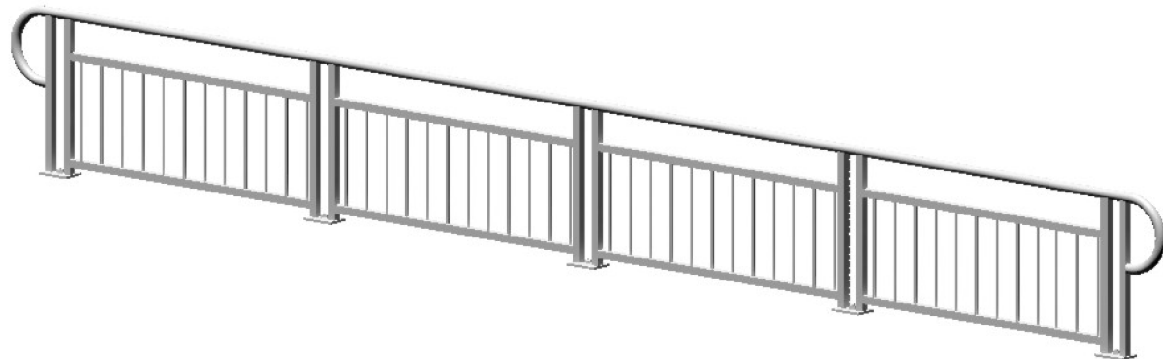
3D VIEW OF RAILING WITH TYPE 1 - PICKET INFILL PANEL (42" Height shown, 48" Height Similar)
