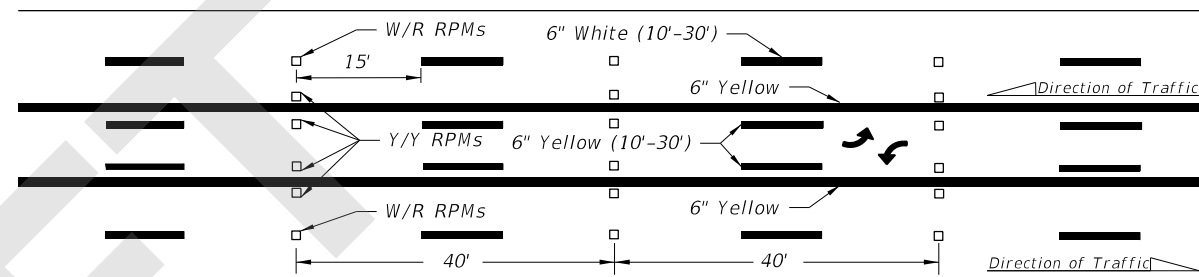
SKIP LINE WITH TWO-WAY LEFT TURN LANE
