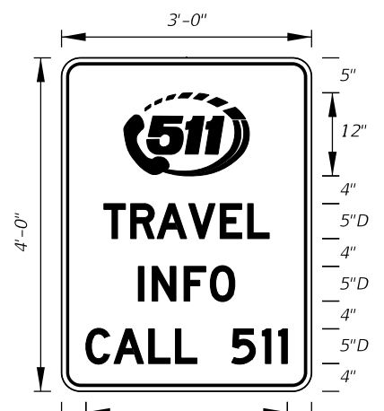
FTP-67-06 3' X 4' 2" Radii 3/4" Border 5" Series D Legend Blue Background White Legend and Border
