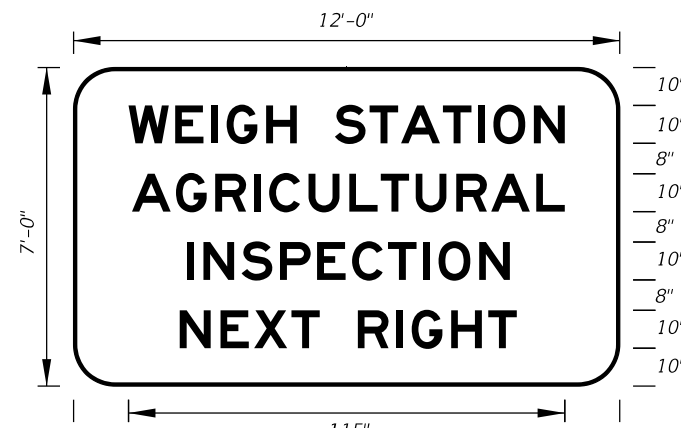
FTP-7A-06 12' X 7' 11" Radii 2" Border 10" Series E Legend Green Background White Legend and Border
