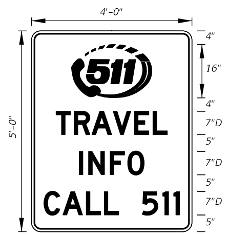
FTP-66-06 4' X 5' 2" Radii 3/4" Border 7" Series D Legend Blue Background White Legend and Border
