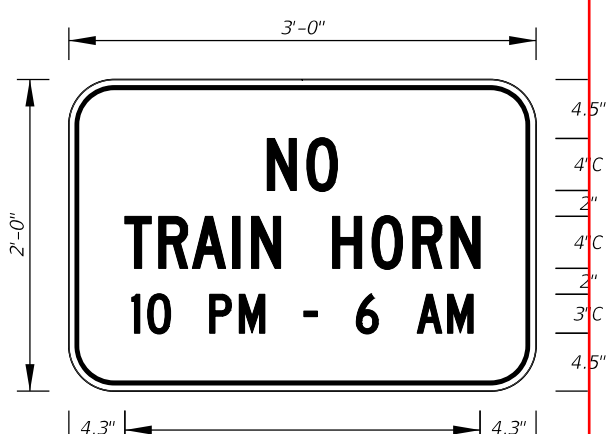
FTP-61-06 3' X 2' 3" Radii 3/4" Border 4" and 3" Series C Legend Yellow Background Black Legend and Border
