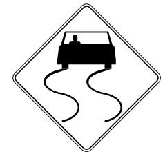
W8-5 SLIPPERY WHEN WET SIGN See Note 11
