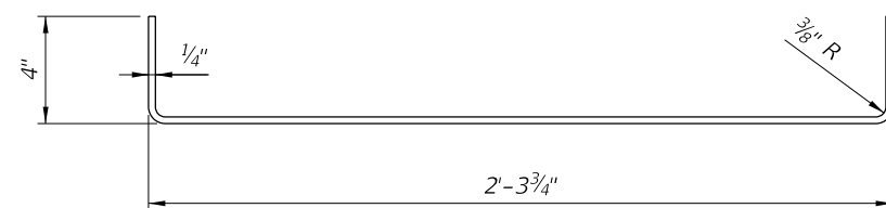
FIXED BEARING KEEPER BAR DETAIL
