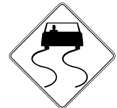
W8-5 SLIPPERY WHEN WET SIGN See Note 11
